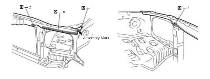
When temporarily installing the new parts, determine the installation position by the assembly mark. Then, measure each part in accordance with the body dimension diagram.
