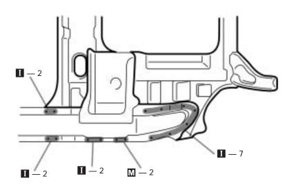
Temporarily install the new parts and measure each part in accordance with the body dimension diagram.
