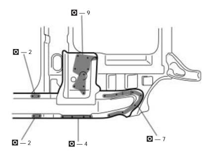
1. Temporarily install the new parts and measure each part in accordance with the body dimension diagram.
