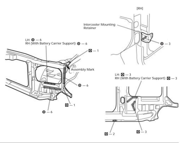
When temporarily installing the new parts, determine the installation position by the assembly mark. Then, measure each part in accordance with the body dimension diagram.
