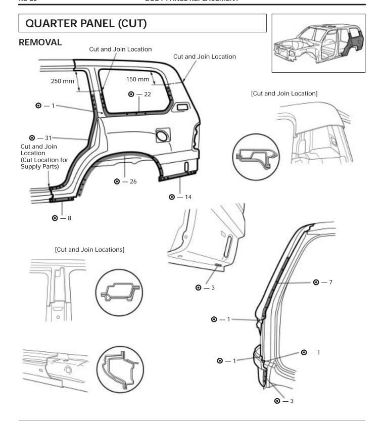
1. Cut and join the parts at the locations as shown above.
