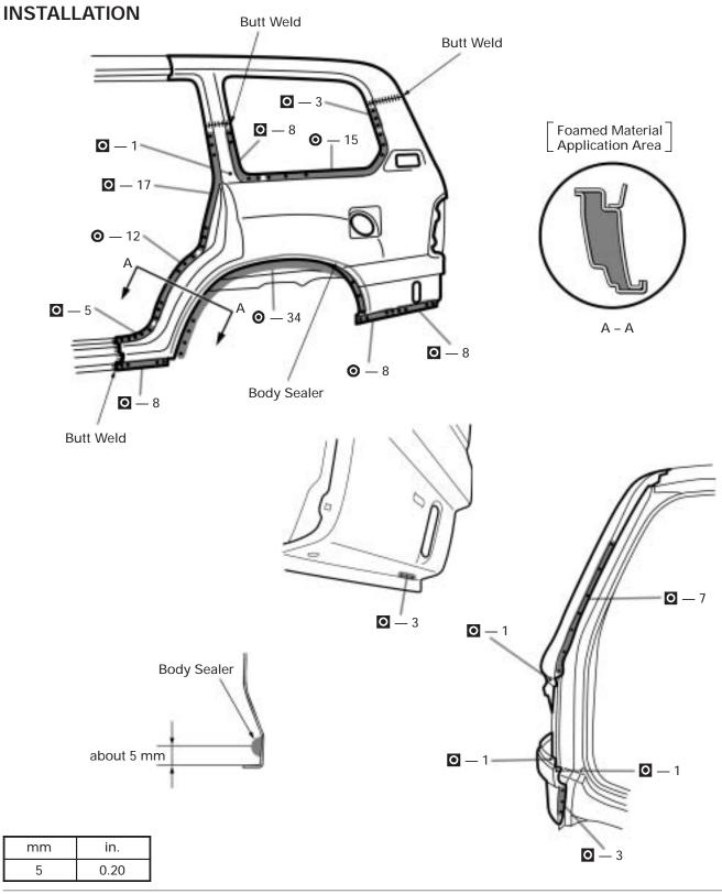
1. Before temporarily installing the new parts, apply body sealer to the wheel arch.
