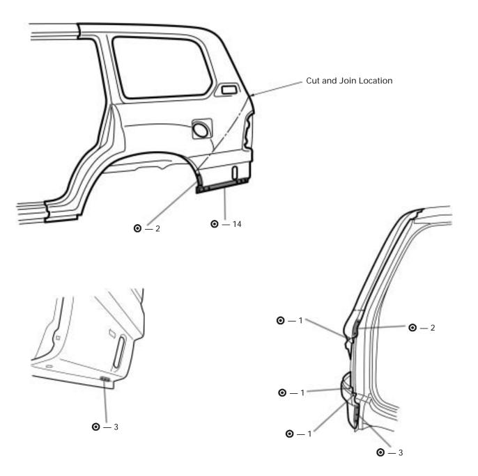
1. Cut and join the parts at the location as shown above.
