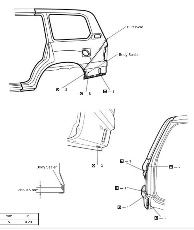
1. Before temporarily installing the new parts, apply body sealer to the wheel arch.
