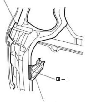
Seat Belt Anchor Reinforcement (3rd Seat Belt Only)
