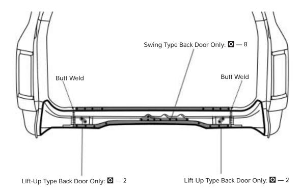
Temporarily install the new parts and check the fit of the tail gate or back door.
