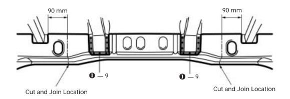
1. Cut and join the parts at the locations as shown above.
