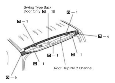
Before temporarily installing the new parts, apply body sealer to the windshield header panel, roof panel reinforcement and back door opening upper frame.
