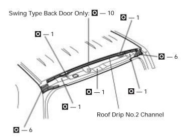
Before temporarily installing the new parts, apply body sealer to the windshield header panel, roof panel reinforcement and back window frame.
