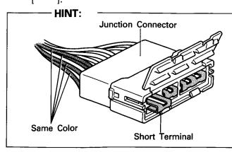
Junction connector (code: J 1 to J53) in this manual include a short terminal which is connected to a number of wire harnesses. Always perform inspection with the short terminal installed. (When installing the wire harnesses, the harnesses can be connected to any position within the short terminal grouping. Accordingly, in other vehicles, the same position in the short terminal may be connected to a wire harness from a different part.)
