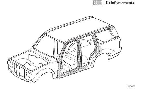
• The side member panel has been integrated in order to realize excellent panel precision and joining rigidity.
