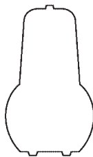
Gasket Cross Section
