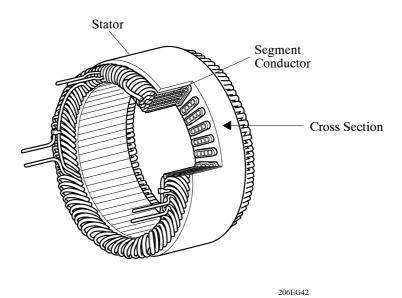
**Stator of Segment Conductor Type Alternator**
