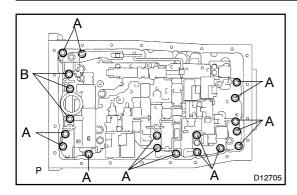
(b) Install the 19 bolts and the valve body.
