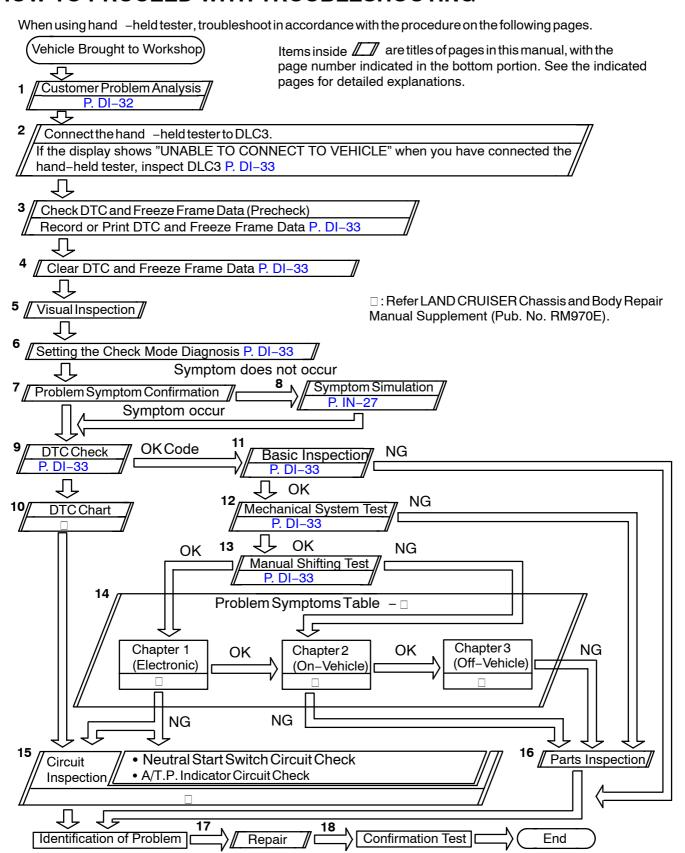
When using hand-held tester, troubleshoot in accordance with the procedure on the following pages.
