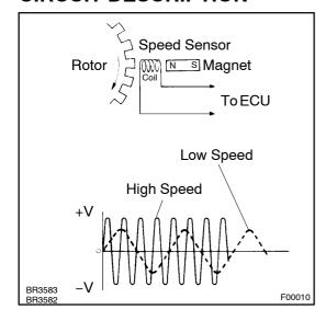
The speed sensor detects wheel speed and sends the appropriate signals to the ECU. These signals are used for control of the ABS control system. The front and rear rotors each have 48 serrations.
