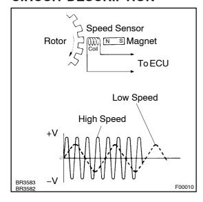
The speed sensor detects wheel speed and sends the appropriate signals to the ECU. These signals are used for control of both the ABS & BA & VSC control system. The front and rear rotors each have 48 serrations.
