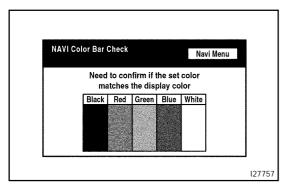
(c) Check each color of the color bar when the "NAVI Color Bar Check" screen is displayed.
