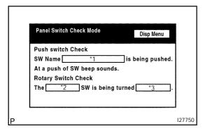
(c) Operate each switch and check that the switch name and condition are correctly displayed.
