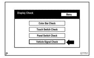
(b) Select "Vehicle Signal Check" from the "Display Check" screen.
