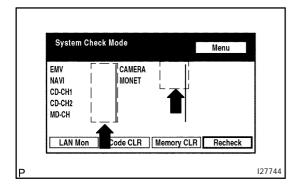
(2) Confirm that all diagnostic codes are "OK" when the check results are displayed.
