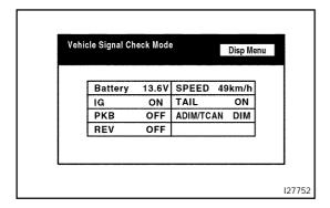
(c) When the "Vehicle Signal Check Mode" screen is displayed, check all the vehicle signal conditions.
