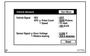
(c) Check all the signals and sensors when vehicle signal information is displayed.
