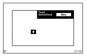
(c) Touch the display anywhere in the open area to perform the check when the "Touch Switch Check" screen is displayed.
