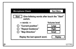
(c) Perform the microphone check by following the directions on the "Microphone Check" screen.
