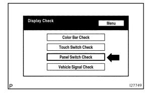
(b) Select "Panel Switch Check" from the "Display Check" screen.
