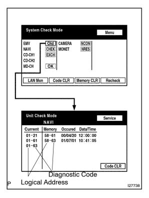
(b) Read the service check result. If all devices report is "EXCH", "CHEK" or "Old" touch the display to check the contents on the "Unit Check Mode" screen and fill them on the customer problem analysis check sheet.
