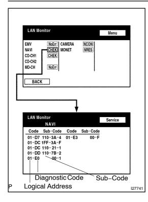
(2) If the result is "CHEK" or "Old" touch this display to check the contents on the "Unit Check Mode" screen and fill them in on the customer problem analysis check sheet.
