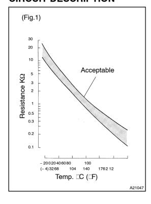
The intake air temperature (IAT) sensor, mounted on the mass air flow (MAF) meter, monitors the intake air temperature. The IAT sensor has a thermistor that varies its resistance depending on the temperature of the intake air. When the air temperature is low, the resistance in the thermistor increases. When the temperature is high, the resistance drops. The variations in resistance are reflected as voltage changes to the engine control ECU terminal.
