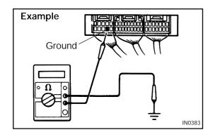
(1) Measure the resistance between the ECU ground terminal and the body ground.
