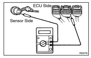
(b) Measure the resistance between the applicable terminals of the connectors.
