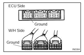
(2) Disconnect the ECU connector. Check for bent ground terminals (on the ECU side and the wire harness side). for Lastly, check the contact pressure.
