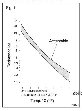
The atmospheric temperature sensor is built into the intake manifold and senses the atmospheric temperature. A thermistor built in the sensor changes the resistance value according to the intake air temperature. The lower the atmospheric temperature, the greater the thermistor resistance value, and the higher the atmospheric temperature, the lower the thermistor resistance value (See Fig. 1).
