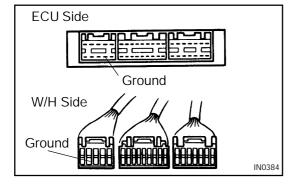
(2) Disconnect the ECU connector, check the ground terminals on the ECU side and the wire harness side for bend and check the contact pressure.
