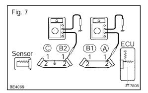
(2) Disconnect connector "B" and measure the resistance between terminal 1 of connector "A" and body ground, and terminal 1 of connector "B2" and body ground.
