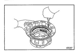
(c) Using a screwdriver, install the snap ring.
