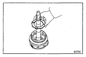
(b) Remove the No.4 thrust washer.
