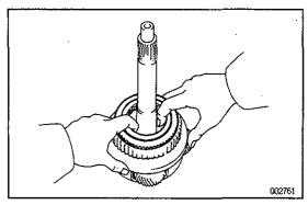
(c) Remove the one—way clutch together with the outer race.
