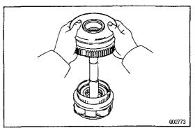
8. INSTALL OVERDRIVE DIRECT CLUTCH ASSEMBLY Install the direct clutch assembly onto the O/D planetary gear.
