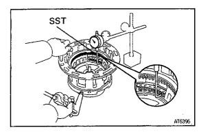
(b) Using SST and a dial indicator, measure the piston stroke by applying and releasing the compressed air 392-785 kPa (4-8 kgf/cm², 57-114 psi) as shown. SST 09350-36010(09350-06120)
