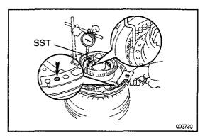
(b) Using SST and a dial indicator, measure the piston stroke by applying and releasing the compressed air 392-785 kPa  $(4-8 \text{ kgf/cm}^2, 57-114 \text{ psi})$  as shown.
