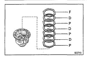
(b) Remove the flange, three discs and three plates.
