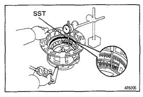
(b) Using SST and a dial indicator, measure the piston stroke by applying and releasing the compressed air 392-785 kPa (4-8 kgf/cm², 57-114 psi)as shown.
