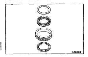
(e) Remove the two retainers and one—way clutch from the outer race.
