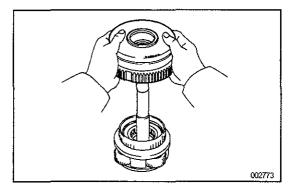
2. REMOVE OVERDRIVE DIRECT CLUTCH ASSEMBLY FROM OVERDRIVE PLANETARY GEAR
