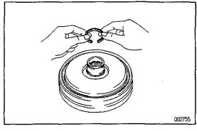
7. REMOVE OIL SEAL RING FROM RING GEAR FLANGE
