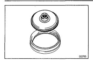
(b) Remove the ring gear flange.
