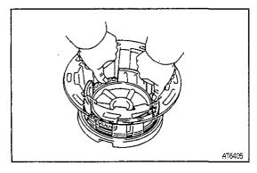
(c) Push in the brake piston into the O/D case with both hands.
