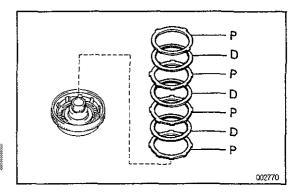
(b) Remove the flange, three discs and three plates.
