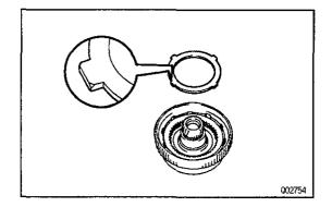
(b) Install the flange, fasing the rounded edge upward.
