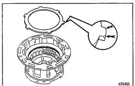
(b) Install the flange, facing the rounded edge upward.
