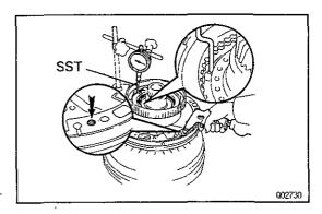
(b) Using SST and a dial indicator, measure the piston stroke by applying and releasing the compressed air 392-785 kPa (4-8kgf/cm², 57-114 psi) as shown. SST 09350-36010(09350-06110)
