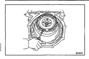
(g) Using a screwdriver, install the snap ring.
