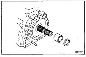
8. INSTALL OUTPUT SHAFT SPACERS
