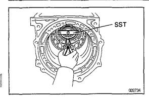
(f) Using snap ring plieres, install the snap ring.
