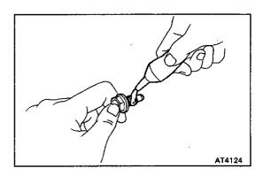
(e) Apply sealant to the threads of the center support set bolts.
