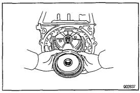
(c) Install the ring gear assembly into the O/D case.
