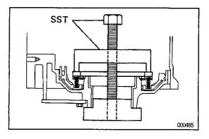
(e) Using SST, compress the return spring. SST 09350-36010(09350-06030)
