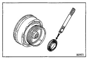
(b) Coat the bearing with petroleum jelly, and install them onto the front clutch hub.
