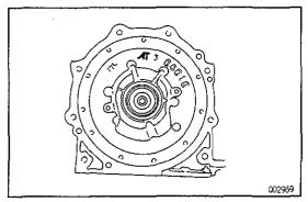
(b) Align the bolt holes of the pump body and transmission case.
