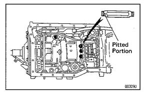
32. INSTALL CENTER SUPPORT APPLY GASKET Install new four gaskets, facing the pitted side toward the transmission case.
