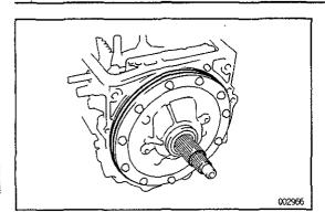
(e) Coat two new O-rings with ATF, and install them to the oil pump body.
