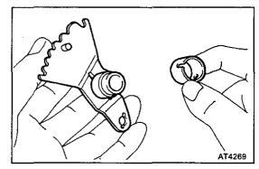
(b) Assemble a new spacer to the manual valve lever.
