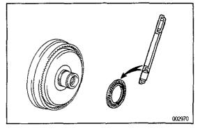
(b) Coat the bearing with petroleum jelly, and install it onto the ring gear flange.
