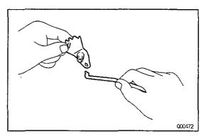
(d) Connect the parking lock rod to the manual valve lever.
