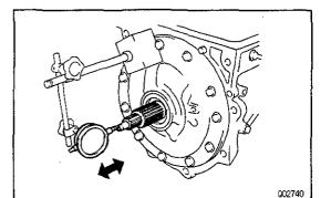
(b) Using a dial indicator, measure the thrust clearance of the input shaft.
