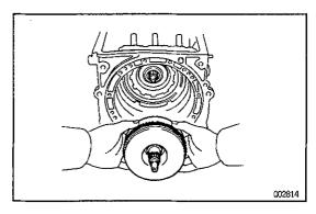
(c) Install the front clutch assembly into the transmission case.
