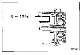
(b) Push the O/D case toward the rear of the transmission by applying a force of 49-98 N (5-10 kgf, 11.0 -22.0 lbf).
