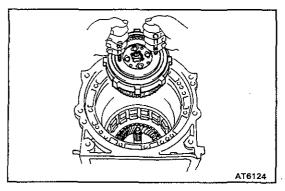
(c) Temporarily install two bolts to the front planetary carrier.
