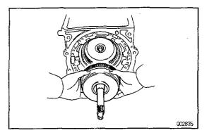
(b) Install the planetary gear, direct clutch and one—way clutch assembly into transmission case.
