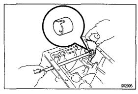
(e) Install the manual valve lever shaft to the transmission case through the manual valve lever.
