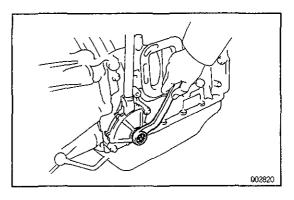
(b) Install the grommet, anew lock washer and the nut.
