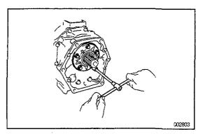
11. INSTALL OUTPUT SHAFT REAR BEARING RETAINER
