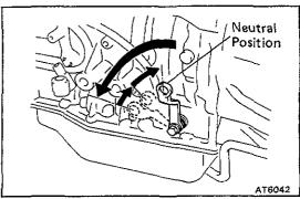
(c) Fully turn the control shaft lever back and return two notches. It is now neutral position.
