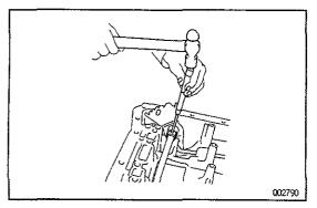
(f) Using a hammer, tap in the pin with the slot at a right angle to the shaft.
