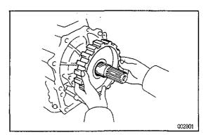
7. INSTALL SPEED SENSOR ROTOR Install the speed sensor rotor onto the output shaft.
