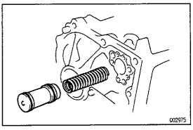
(b) Install the spring and accumulator piston into the bore of the transmission case.
