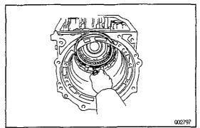
(j) Install the snap ring.HINT: Be sure the end of the snap ring is not aligned with the cutout portion of the transmission case.
