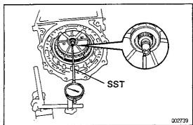
(c) Using SST and a dial indicator, measure the thrust clearance of the input shaft.
