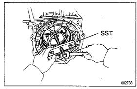
(e) Using SST, remove the O/D case assembly. SST 09350-36010(09350-06140)
