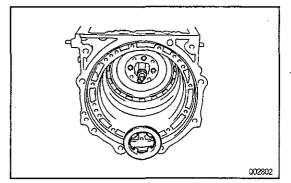
(h) Coat the thrust washer with petroleum jelly, and install it onto the front planetary carrier.
