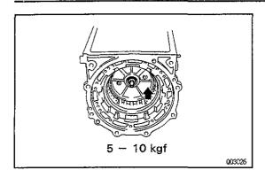
(b) Push the center support toward the rear of the transmission by applying a force of 49-89 N (5-10 kgf, 11.0-22.0 lbf), then pull with the same amount of force.
