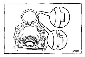
(i) Install the flange, facing the rounded edge outward. HINT: If the flange is step-edged, install the flange with the step-edge, facing inward.
