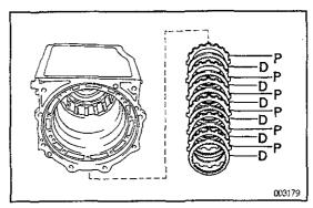
(h) Install the six plates and six discs in order:P = Plate D = Disc
