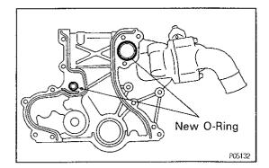
(c) Place two new O-ring in position on the timing chain cover.
