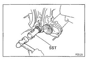
HINT: If necessary, install the gear with SST. SST 09636-20010
