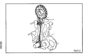
(c) Tie the timing chain with a cords as shown in the illustration and make sure it doesn't come loose.
