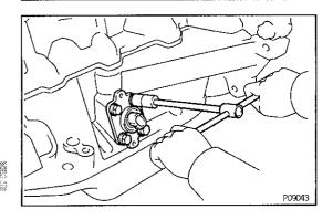
(b) Install the level sensor with the four bolts.
