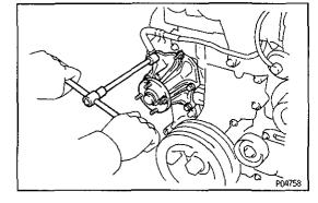
(d) Remove the four bolts, two nuts, water pump and gasket.
