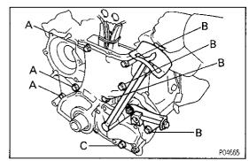
(e) Install the oil pump and drive belt adjusting bar with the nine bolts and two nuts.
