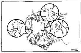
(b) Remove the timing chain cover by prying the portions between the cylinder block and timing chain cover with a screwdriver.
