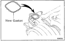
(c) Install a new gasket in position.
