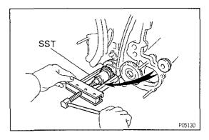
HINT: If necessary, remove the gear with SST. SST 09213-36020, 09950-20017
