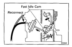
(e) Reconnect the vacuum hose, and check that the choke linkage moves, and that the fast idle cam is released to the 4th step.
