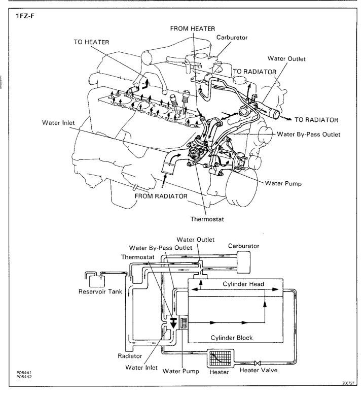
The cooling system is composed of the water jacket (inside the cylinder block and cylinder head), radiator, water pump, thermostat, cooling fan, hoses and other components.
