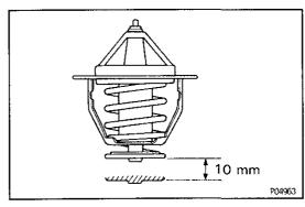
(c) Check the valve lift.
