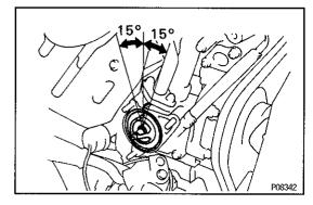
(b) Align the jiggle valve of the thermostat with the protrusion of the water inlet housing, and insert the thermostat in the water inlet housing.
