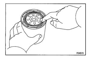
(c) Apply clean engine oil to the gasket of a new oil filter.
