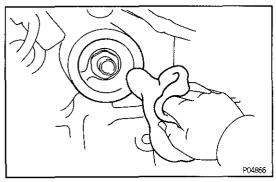
(b) Check and clean the oil filter installation surface.
