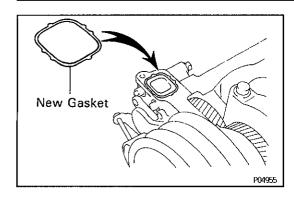
(c) Install a new gasket in position.
