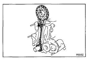
(c) Tie the timing chain with a cord as shown in the illustration and make sure it doesn't come loose.
