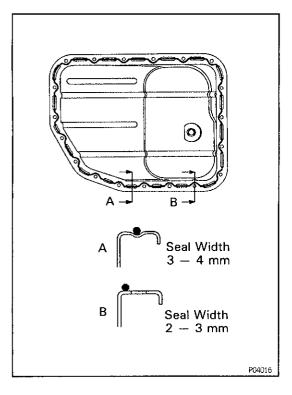
Install a nozzle that has been cut to a 2 - 3 mm (0.08 - 0.12 in.) opening or 3 - 4 mm (0.012 - 0.016 in.) opening.
