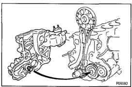
(d) Engage the gear of the oil pump drive rotor with the gear of the oil pump drive gear, and slide the oil pump.
