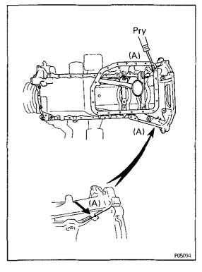
(b) Remove the No.1 oil pan by prying the portions (A) between the cylinder block and No.1 oil pan with a screwdriver.
