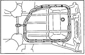
(c) Install the No.2 oil pan with the 17 bolts and two nuts.
