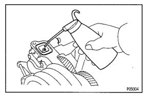
(d) Pour in approximately 15 cm<sup>3</sup> (0.9 cu in.) of engine oil in position.
