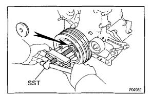
HINT: If necessary, remove the pulley with SST. SST 09213-60017 (09213-00020, 09213-00030, 09213-00060), 09950-20017
