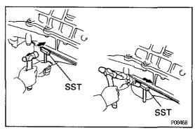
(b) Insert the blade of SST between the No.1 and No.2 oil pans, cut off applied sealer and remove the No.2 oil pan.
