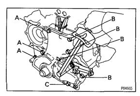
(e) Install the oil pump and drive belt adjusting bar with the nine bolts and two nuts.
