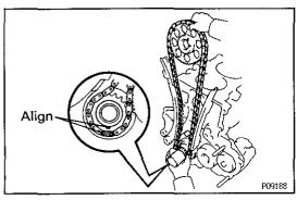
(b) Install the timing chain on the crankshaft timing gear with the other bright link aligned with the timing mark on the crankshaft timing gear.
