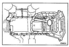
(e) Install the No.1 oil pan with the 21 bolts and two nuts.
