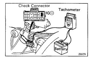
2. With a tachometer connected to the system, connect the test probe of the tachometer to the IG⊖ of the check connector.
