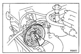
(b) Check that the distributor rotor direction is as shown. If not, turn the crankshaft pulley one complete revolution.
