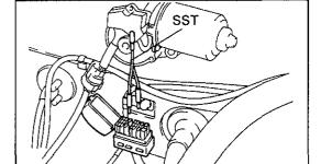
(e) Remove SST from the data link connector 1. SST 09843-18020
