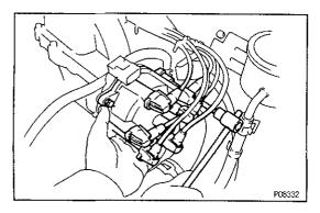
3. REMOVE DISTRIBUTOR CAP WITHOUT DISCONNECTING HIGH-TENSION CORDS
