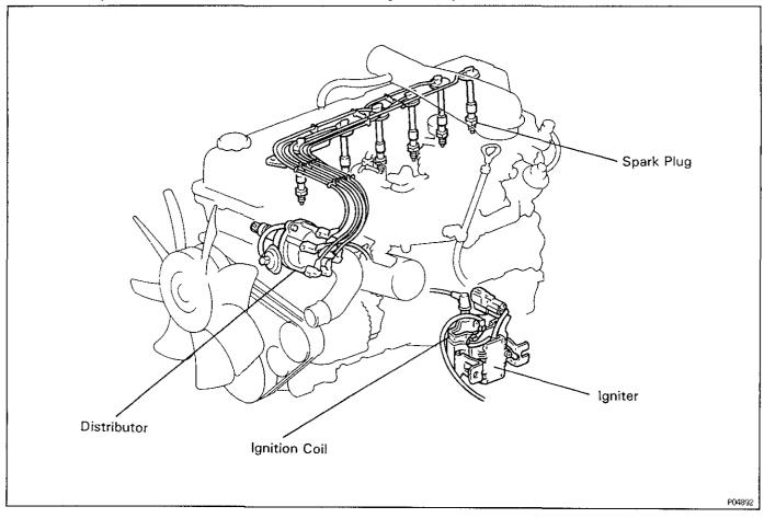
This ignition system is comprised of a distributor, ignition coil, igniter, spark plugs and other componentes.
