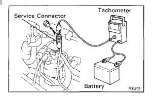
2. With a tachometer connected to the system, connect the test probe of the tachometer to the service connector from the igniter.
