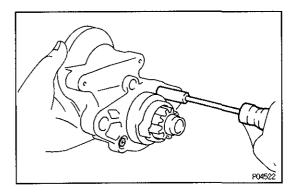
(d) Assemble the starter housing and magnetic switch assembly and install the two screws.
