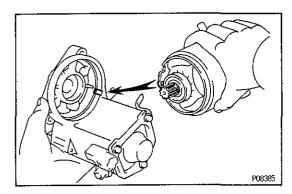
(b) Align the protrusion of the field frame with the cutout of the magnetic switch.
