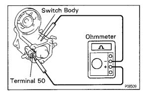
2. PERFORM HOLD—IN COIL OPEN CIRCUIT TEST
