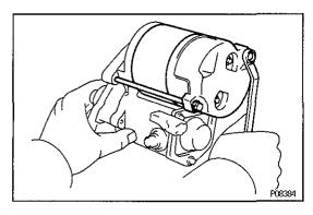
(c) Install the field frame and armature assembly with the two through bolts.
