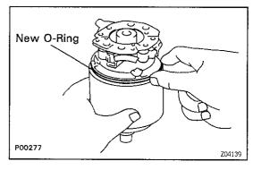
(c) Place a new O-ring in position on the field frame.
