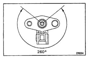
HINT: The idle mixture adjusting screw can be tightened through on angle of 260°.
