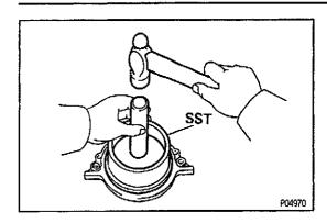
(b) Using SST and a hammer, tap in a new oil seal until its surface is flush with the rear oil seal edge. SST 09223-15030, 09950-70010 (09951-07150) NOTICE: Do not let foreign matter get onto the lip of the oil seal.
