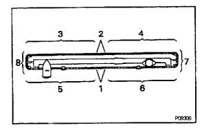
(b) Stake the claws of the tank plates with SST in the numerical order shown in the illustration.
