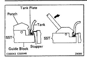
NOTICE: If the bottom of the core plate is staked with the SST on the guide block stopper, it may result in water leakage.
