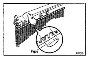
• Do not stake the areas protruding around the pipes.
