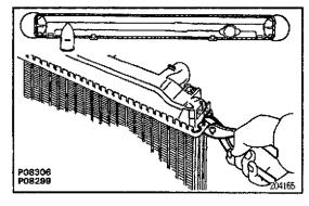
The points shown in the illustration cannot be staked with the SST. Use pliers and be careful not to damage the core plates.
