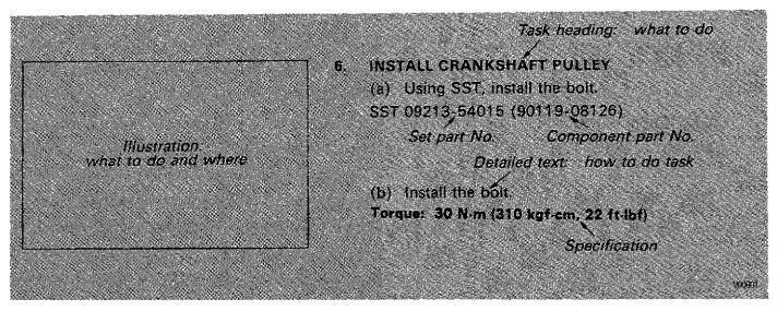
This format provides the experienced technician with a FAST TRACK to the information needed. The upper case task heading can be read at a glance when necessary, and the text below it provides detailed information. Important specifications and warnings always stand out in bold type.
