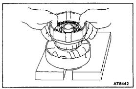
(b) Being careful not to damage the O-rings, press the clutch piston into the forward clutch drum with both hands.
