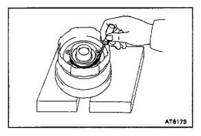
2. INSTALL NEW O-RING TO FORWARD CLUTCH DRUM
