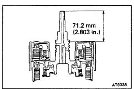
(d) Check that the distance from the direct clutch end to the forward clutch end is 71.2 mm (2.803 in.). If the distance is less than the above value, parts may have been assembled incorrectly, check and reassemble again.
