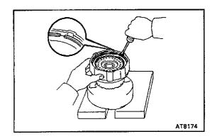
(c) Install the snap ring with a screwdriver. Be sure the end gap of the snap ring is not aligned with the cutout portion of the forward clutch drum.
