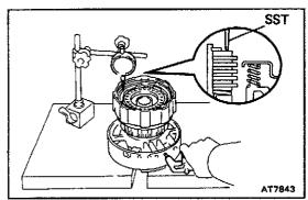
3. CHECK PACK CLEARANCE OF FORWARD CLUTCH Using SST and a dial indicator, measure the forward clutch piston stroke while applying and releasing compressed air (392-785 kPa, 4-8 kgf/cm², 57-114 psi).
