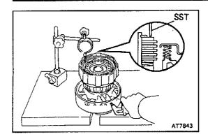
CHECK PACK CLEARANCE OF FORWARD CLUTCH Using SST and a dial indicator, measure the forward clutch piston stroke while applying and releasing com-
