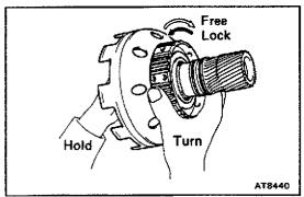
6. CHECK OPERATION OF NO.1 ONE—WAY CLUTCH Hold the planetary sun gear and turn the 2nd brake hub. Check that the 2nd brake hub must be able to turn freely clockwise and locks counterclockwise.
