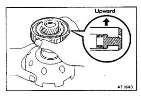
5. INSTALL ASSEMBLED NO.1 ONE—WAY CLUTCH AND 2 ND BRAKE HUB ONTO PLANETARY SUN GEAR
