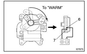
(2) Connect the positive (+) lead from the battery to terminal 7 and negative (-) lead to terminal 6, then check that the arm tuns to "WARM" side smoothly. If operations are not as specified, replace the servomotor.
