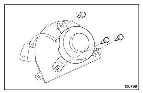
(c) Remove the 3 screws and motor.
