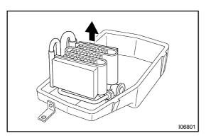
(b) Remove the evaporator with expansion valve.
