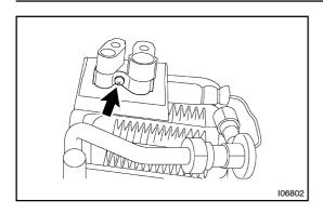
(c) Remove the screw and piping clamp.
