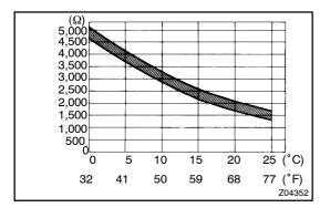
(b) Compare the 2 readings on the chart. If resistance value is not as specified, replace the thermistor.
