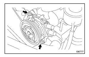
(c) Remove the 2 bolts and viscous heater.
