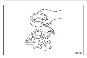
(c) Remove the stator.
