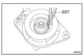
(b) Using SST, remove the snap ring. SST 07114 -84020
