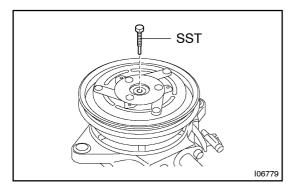
(b) Install SST on the pressure plate. SST 07112 -66040
