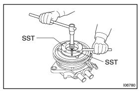
(c) Using SST and a socket wrench, remove the pressure plate.
