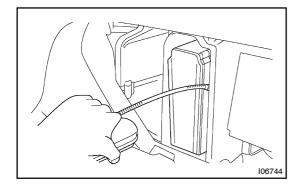
(c) Using a gas leak detector, check for leakage of refrigerant
