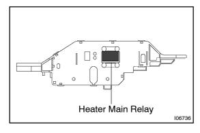
(e) Remove the heater main relay from junction block.
